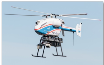
Fig. 1: DLR's autonomous superAR-TIS equipped with optical navigation.
