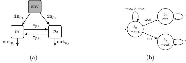
Fig. 3: The architecture used for our experiments in (a) where the number outputs, inputs, and communication channels can vary. Figure 3b shows the implementation of process b for its bit transmission component specification.
