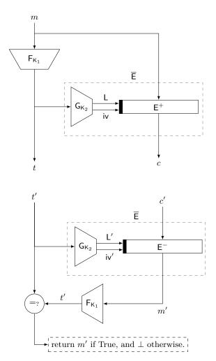
Figure 3.1: Encryption (top) and decryption (bottom) algorithms in MTProto-G. The dashed rectangle represents the IV-based encryption scheme  $\overline{E}$ .
