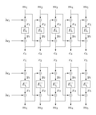
Figure 3.4: IGE encryption (top) and decryption (bottom) algorithms.
