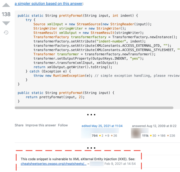
Figure 2: A Stack Overflow answer post with comments and change history. The original post was created on Aug 12, 2009, and the code was edited on Feb 23, 2011. Almost ten years later, a comment (dashed line) points out an XXE vulnerability, which led to a code revision (see Figure 3).
