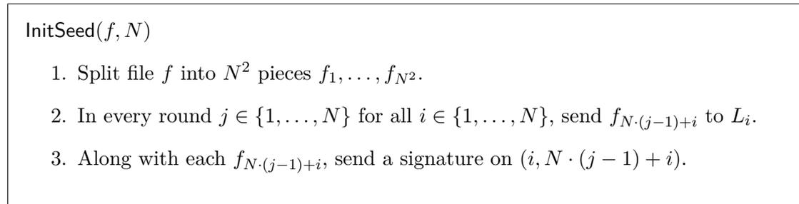
Figure 3.1: Algorithm for the seeder describing whom to upload pieces to.
