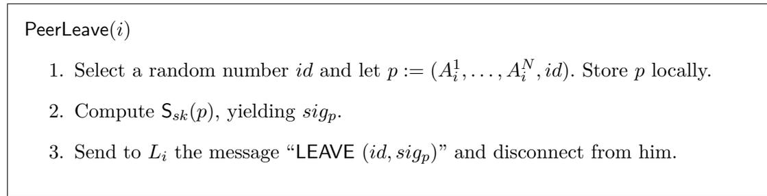
Figure 4.2: Tracker’s algorithm invoked when a leecher wants to leave and rejoin later
