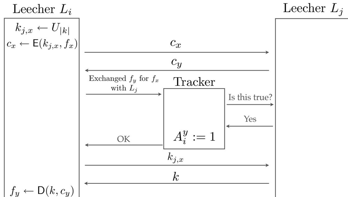
Figure 4.5: Piece exchange protocol for leecher  $L_i$
